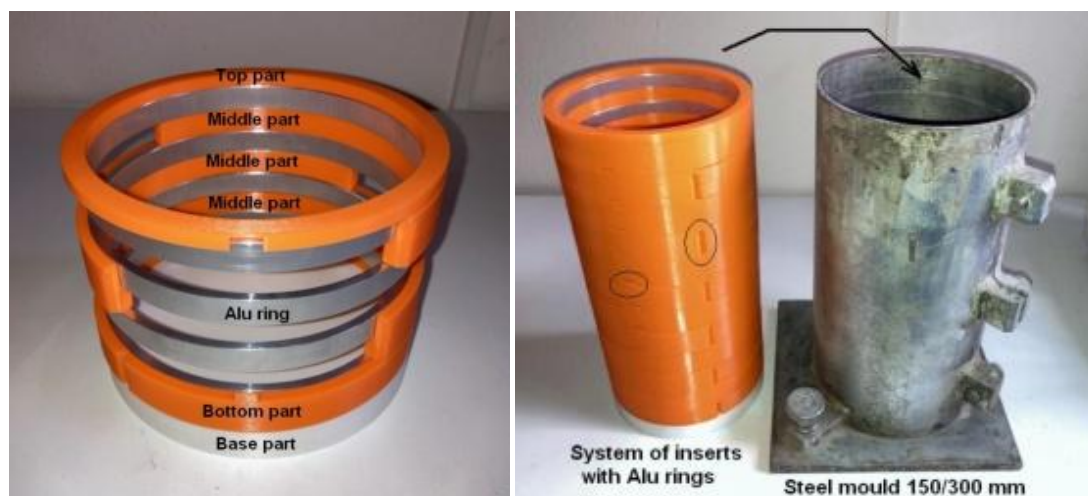
Fig. 12: Demonstration of the principle of assembling individual parts (inserts) and aluminum rings (left). The individual layers are made up of two parts with locks so that they can be removed during demolding. The result is a "custom mold inserted into a standard mold" (right).
